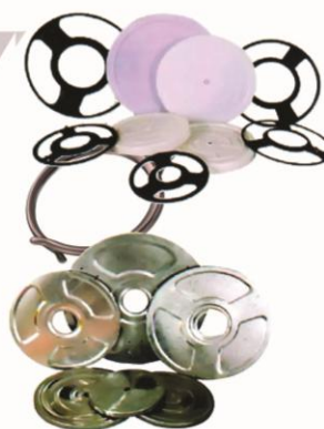
Galvanized Iron Bottom Plate Of 9" To 40" Dai Can These Bottom Plates Are Made From Deep Drawing Quality Gi Sheets Which Are Equidistansy Embossed To Enhance The Overall Strength And To Avoid Any Deformation.
